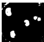
Figure 6-22 Thresholded "S" plane of the image
