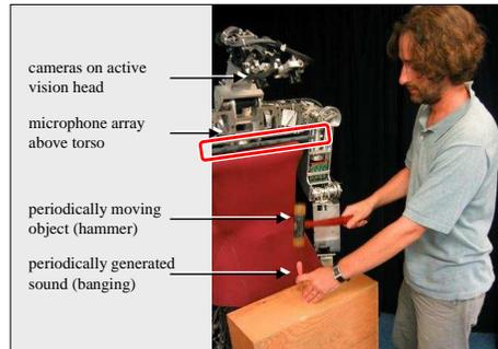
Figure 1: The experimental platform. The humanoid robot Cog [2] is equipped with cameras in an active vision head, and a microphone array across the torso. A human demonstrates some repetitive action to the robot, such as using a hammer.
