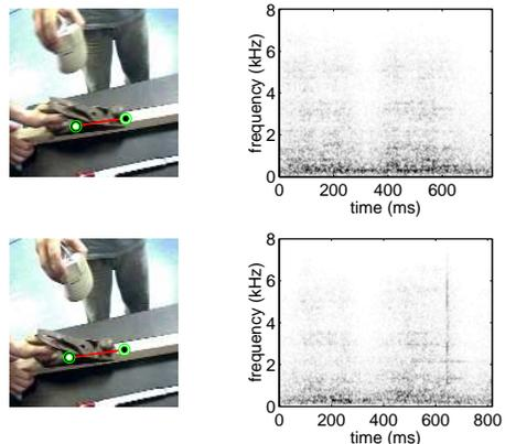
Figure 7: An experiment in which a plane is being pushed across wood while a mouse is shaken in the background. Shown are the highest quality acoustic matches for this sound (right) and the object with which they correspond (left). Matches against the mouse are much lower and below threshold.
