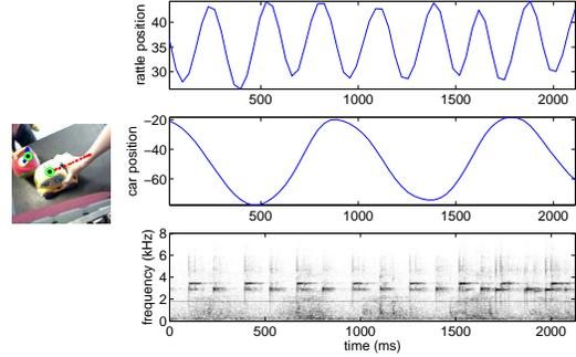
Figure 5: The car and the cube, both moving, both making noise. The line overlaid on the spectrogram (bottom) shows the cutoff determined automatically between the high-pitched bell in the cube and the low-pitched rolling sound of the car. A spectrogram of the car alone can be seen on Figure 3. The frequencies of both visual signals are half those of the audio signals.
