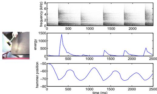
Figure 2: Audio and visual information for a hammer hitting a table. The robot monitors the spectrum of the sound signal (the top graph shows the complete spectrogram, the middle graph shows the overall energy signal) while tracking the trajectory of objects visible to its camera (bottom).
