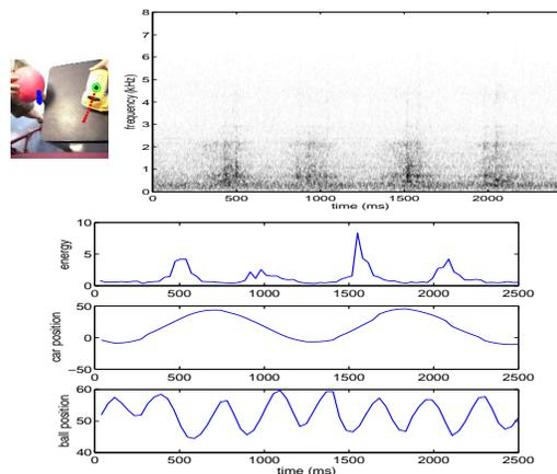
Figure 3: The top left image shows a car and a ball moving simultaneously, with their trajectories overlaid. The spectrogram during this event is shown to the right. Sound is only generated by the rolling car – the ball is silent. A circle is placed on the object (car) with which the sound is bound. The sound energy and the visual displacements of the objects are given.
