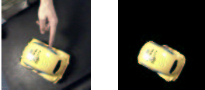
Figure 6-4: The segmentation algorithm will work for human poking operations, if the robot is fixating the object the human pokes. The robot can be made to fixate objects by bringing its attention to it by any of the means discussed in Chapter 8.
