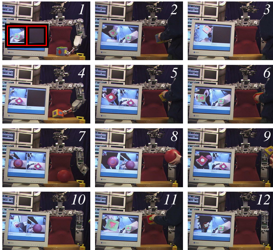
Fig. 13. This figure shows stills from a three-minute interaction with Cog. The area of the first frame highlighted with a square shows the state of the robot – the left box gives the view from the robot’s camera, the right shows an image it associates with the current view. Initially the robot is not familiar with any objects, so the right box is empty. It is presented with the cube, and pokes it (first frame). Then, if shown the cube again, it recognizes it (this recognition is evidenced by showing an image recorded from when the object was poked). If the cube is turned to another side, the robot no longer recognizes it (third frame). If that side of the cube is presented to the robot to poke (fourth frame), it can then recognize it (fifth frame) and differentiate it from the green side (sixth frame). If it confuses another object with what it has already seen, such as the ball in the seventh frame, this is easily to fix by poking (eighth, ninth frames). The final three frames show the invariance of the recognition system to scale.
