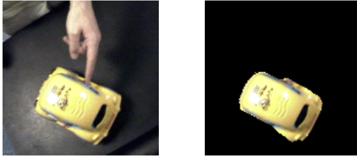
Figure 12. The segmentation algorithm will work for human poking operations, if the robot is fixating the object the human pokes. The robot’s attention system makes this a simple condition to satisfy.
