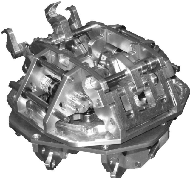
Fig. 3. The ATRON module, 11cm in diameter, without electronics and batteries.
