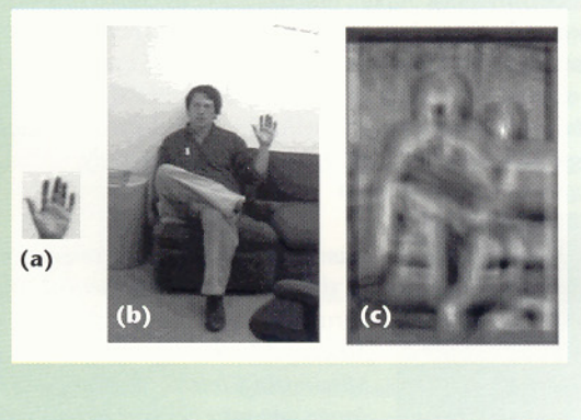
E (a) Stored hand template. (b) Image to be analyzed. (c) Normalized correlation values at each pixel. The bright spot of the normalized correlation indicates the position of the best match.
