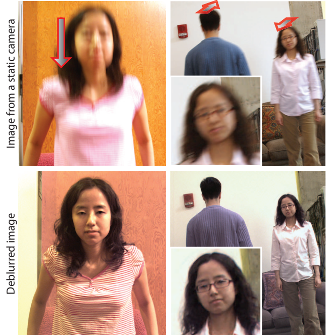
Figure 6: Images taken with a synchronized static camera and deblurred images from the orthogonal parabolic camera. Images from a static camera with 500ms exposure are shown for reference. Arrows on reference images show the direction and magnitude of motion.
