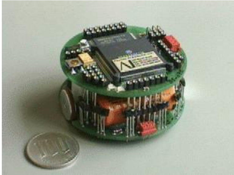
Figure 5-3: The Khepera is small enough, and constrained to such simple environments, that “reality gap” has been reduced to trivial proportions.
