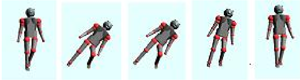
Fig. 8.2 – Balance recovery from lateral disturbance using spin angular momentum.
