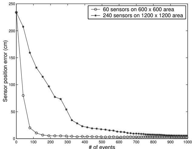
**Fig. 10.** Effect of network size on SLAT localization accuracy.
