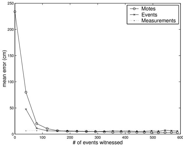
**Fig. 4.** SLAT estimate error vs. number of observed events. In this simulation, 60 sensors are spread over a 600 cm x 600 cm area. Simulated targets move along continuous paths through the network producing events as they move. Each mark on the graph represents the status of the network after an iteration of the SLAT algorithm. Error is measured relative to ground truth. As predicted, SLAT's localization estimate improves over time; this drives the improvement in event error.
