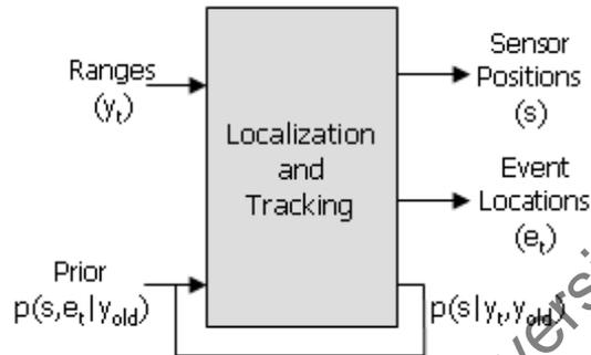
**Fig. 1.** The SLAT architecture. Given a Gaussian prior distribution and a collection of ranges to some events, SLAT produces an estimate of the sensors' positions, an estimate of the events' locations, and a more informative Gaussian prior for use with future computations.
