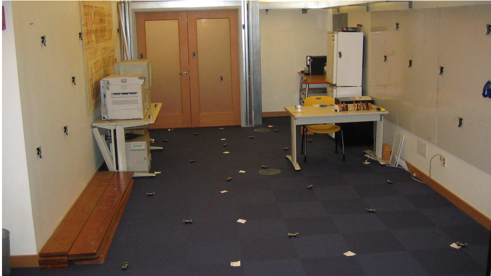
Figure 6: Environment used for initial 3d localization experiments. LaSLAT localized sensors to within 7 cm.
