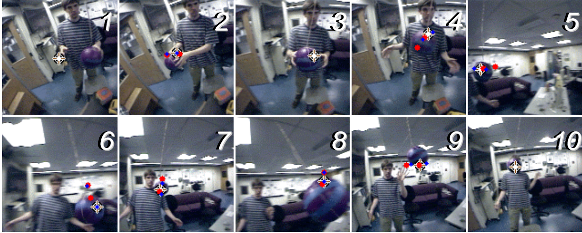
Figure 8-8: The tracking system has an inbuilt preference for moving objects. This means that if the robot is staring at something, and you want to bring the robot's attention to it, then you can simply move the object in front of the robot (frames 1 to 2). This figure shows frames from a 9 second sequence of the robot (Cog) tracking a rapidly moving ball suspended from the ceiling by elastic until it crashes into the author's face. The crosshair shows the current tracked target. Notice the wide range of motion (compare frames 1, 5, 10) and distance to the ball (compare frames 7 and 8) over this short sequence. The tracker continually looks several pixels forward and backward along its direction of motion and then shifts to whichever location is moving most rapidly. This keeps the tracker on the target, although it will not stay locked to a specific part of the target.
