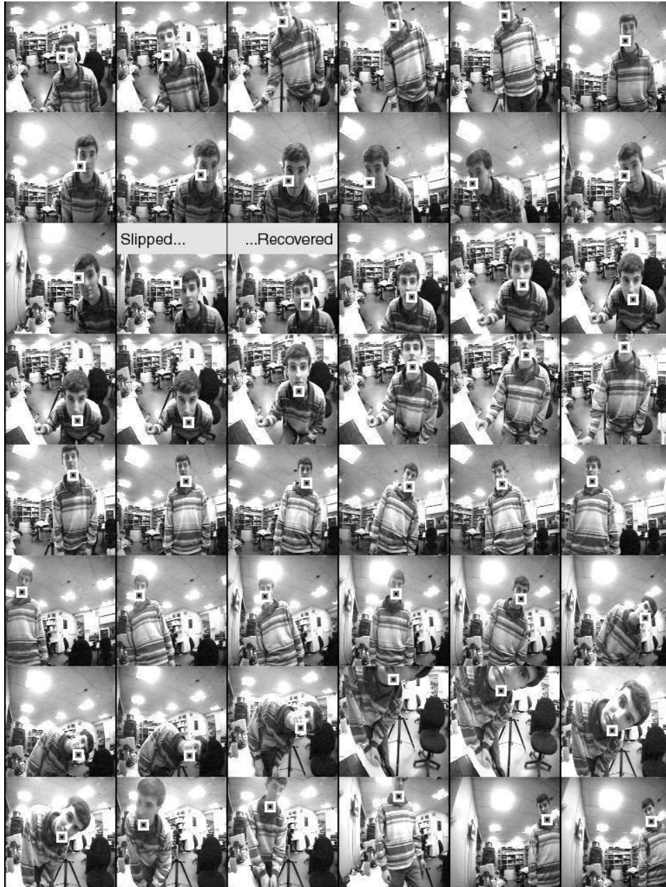
Figure 8-9: Behavior of the tracker over a longer period (on Kismet). Frames are taken at one second intervals. The white squares indicates the position of the target. The target is not centered in the images since they were taken from a camera fixed with respect to the head. On the third row, the face slips away from the tracker, but it is immediately reacquired through the attention system. The images are taken from a three minute session during which the tracker slipped five times. This is typical performance for faces, which tend not to move too rapidly.
