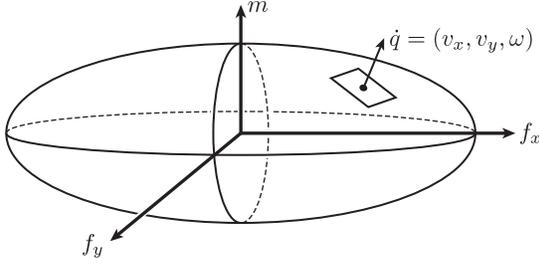
Fig. 5. Ellipsoidal approximation of the limit surface  $F(f_x, f_y, m) = 0$ . The lengths of the major axis of the ellipsoid are  $f_{\max}$  along  $f_x$  and  $f_y$ , and  $m_{\max}$  along  $m$ . Any point on the surface of the ellipsoid represents a total frictional load on a sliding object. Its resulting velocity  $\dot{q}$  must be along the gradient  $\nabla F(f_x, f_y, m)$ .
