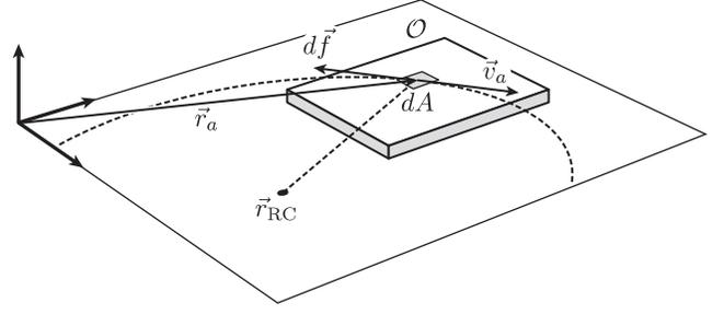
Fig. 4. Integration of infinitesimal friction force to compute the total frictional load between an object  $\mathcal{O}$  and its support. If the instantaneous center of rotation of the object is at  $\vec{r}_{RC}$ , a point  $\vec{r}_a$  with differential support  $dA$  on the support will move with velocity  $\vec{v}_a$  and will contribute with an infinitesimal friction force  $d\vec{f}$  that opposes  $\vec{v}_a$ .
