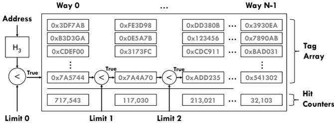
Figure 9: GMONs enhance UMONs with varying sampling rate across ways, controlled with per-way *limit registers*.
