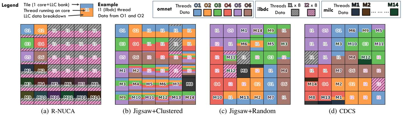
Figure 1: Case study: 36-tile CMP with a mix of single- and multi-threaded workloads (omnet $\times$ 6, milc $\times$ 14, 8-thread ilbdc $\times$ 2) under different NUCA organizations and thread placement schemes. Threads are labeled and data is colored by process.
