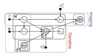
Fig. 2. Graphical representation of the generative model. Hollow circles denote random variables, solid circles represent hyper-parameters, and shaded circles represent observed variables. The rectangle containing  $\mathbf{v}_m$  represents deterministic variables to be estimated. The plates indicate conditionally independent instantiations.
