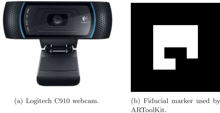
Figure 2: Hardware for the localization system consisting of one or more webcams used to extract the pose of multiple black-and-white fiducial markers.
