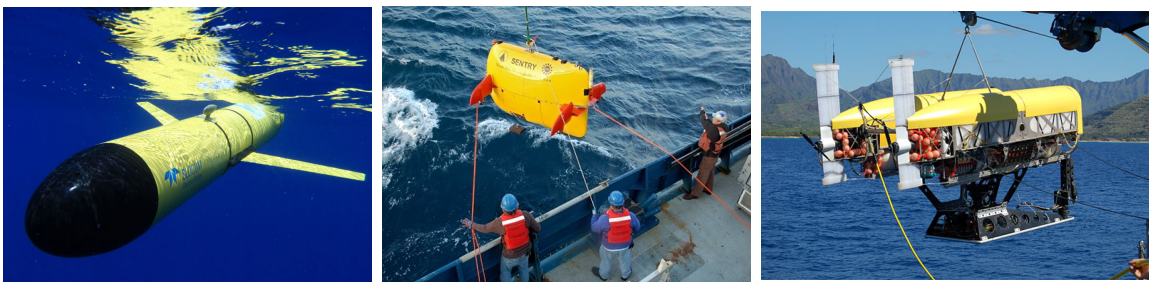
(a) Slocum glider. (b) Sentry autonomous underwater vehicle. (c) Nereus remotely-operated vehicle.
