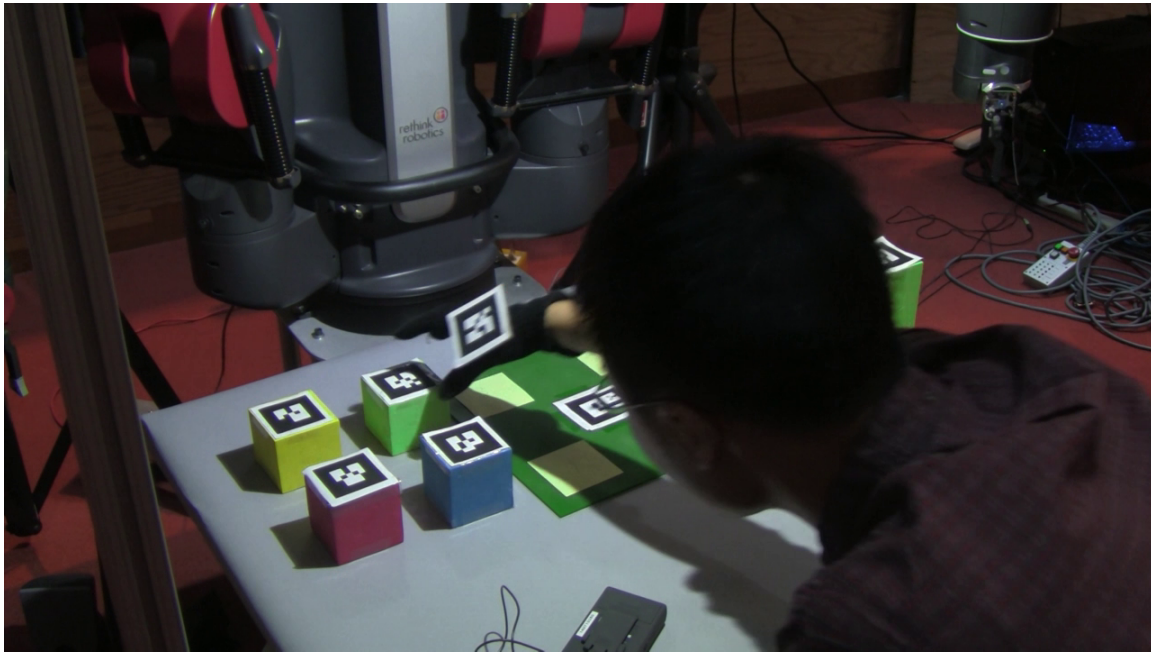
Figure 7-15: Simple collaborative pick-and-place task between the Baxter and a human coworker.
