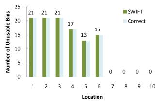
**Figure 12: Adaptive Sensing is Robust:** At each location, SWIFT finds the correct unusable bins, *i.e.* those that interfere with 802.11a.
