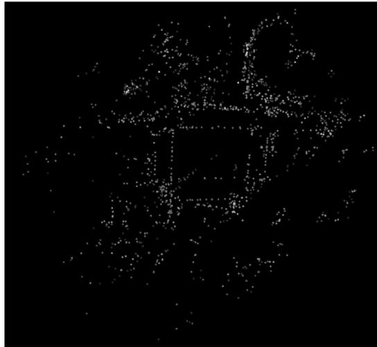
Figure 5.36: Bundler reconstruction of CLIF Intersection - Ortho view (1,715 points)
