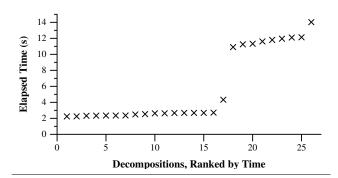
**Figure 13.** Elapsed time for IpCap to  $\log 3 \times 10^5$  random packets for 26 decompositions up to size 4 generated by the auto-tuner, ranked by elapsed time. The 58 decompositions not shown did not complete within 30 seconds.
