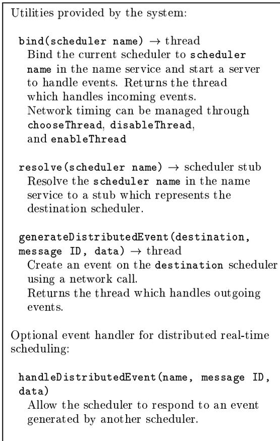
**Figure 4: Distributed real-time thread and event support**
