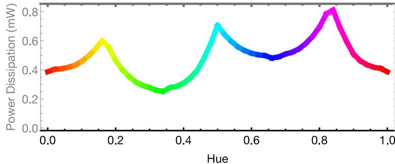
Figure 2. The power dissipation of OLED displays varies with hue (which wraps on  $[0, 1]$ ). The data shown are from hardware measurements on a representative OLED display. Points in the plot represent power dissipation at a given hue. The line joining the points is colored to show the hue variation.
