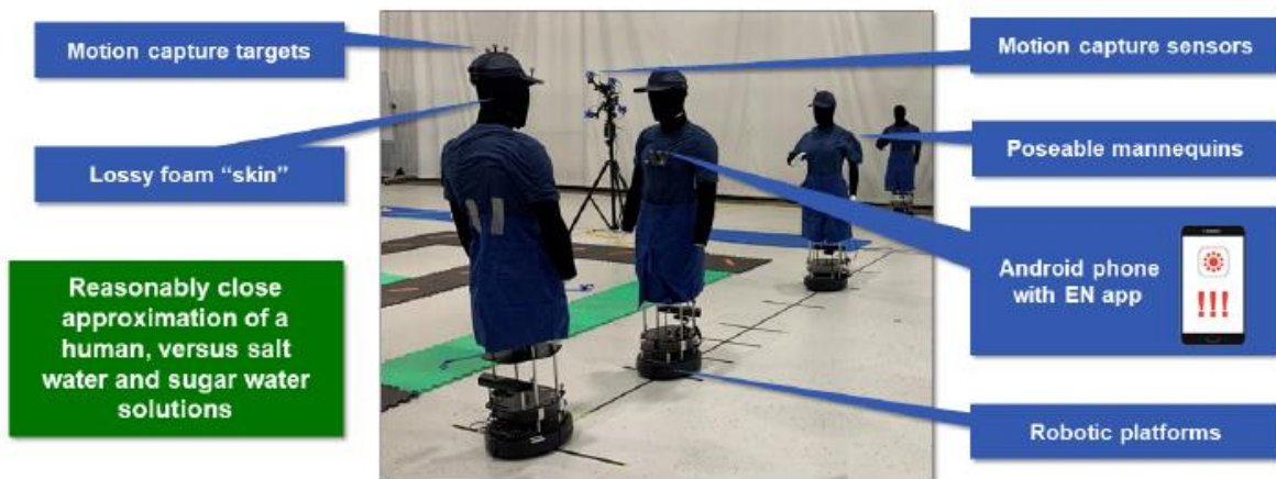
Figure 3. Data collection hardware, software, and infrastructure at MIT Lincoln Laboratory.
