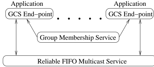
Figure 1: The client-server architecture: GCS end-points using an external membership service. Arrows represent interaction between GCS end-points and underlying services.
