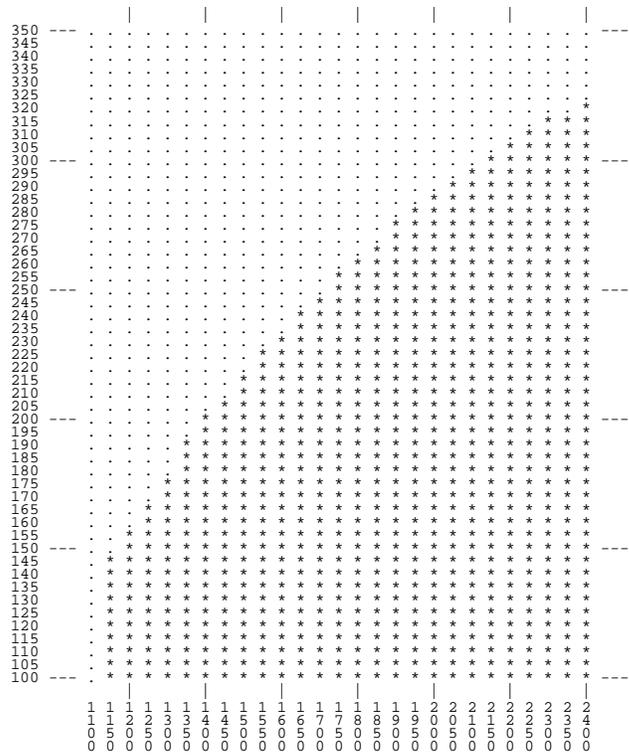
Figure 6-11: Shmoo plot for Scale chip operating in the on-chip RAM testing mode. The horizontal axis plots supply voltage in mV, and the vertical axis plots frequency in MHz. A “\*” indicates that the chip functioned correctly at that operating point, and a “.” indicates that the chip failed.
