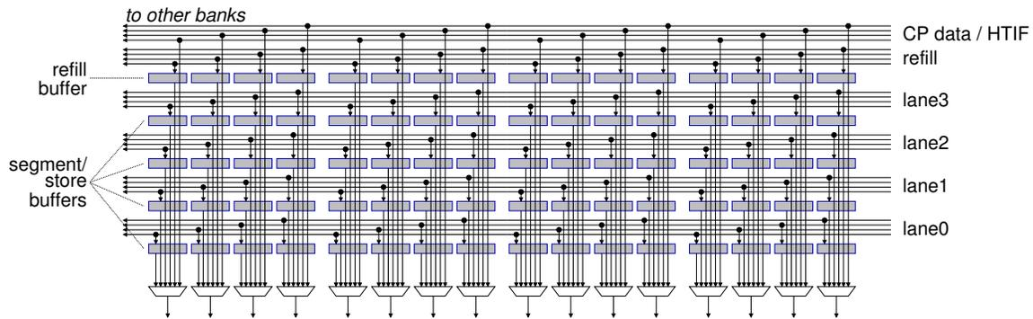
Figure 5-26: Write crossbar. Only one bank is shown, but the horizontal wires extend to all four banks and the crossbar in each is identical. All wires in the figure are 8-bits wide. The 16 crossbar muxes send 128-bits of write data to the bank.
