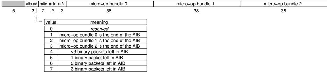
Figure 5-6: Binary instruction packet encoding. Three micro-op bundles are packed together in a 128-bit word. The `m0c`, `m1c`, and `m2c` fields indicate which cluster each micro-op bundle is for. The `aibend` field indicates how many packets remain in the AIB, or which micro-bundle slot in this packet is the end of the AIB.
