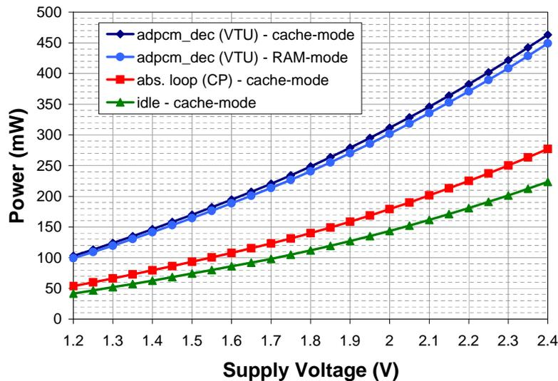
Figure 6-14: Chip power consumption versus supply voltage at 100 MHz. Results are shown for idle (clock only), the control processor absolute-value test program, and the VTU `adpcm_dec` test program. The cache is enabled for the idle and CP results. For the VTU program, results are shown for both the on-chip RAM operating mode and the cache operating mode.
