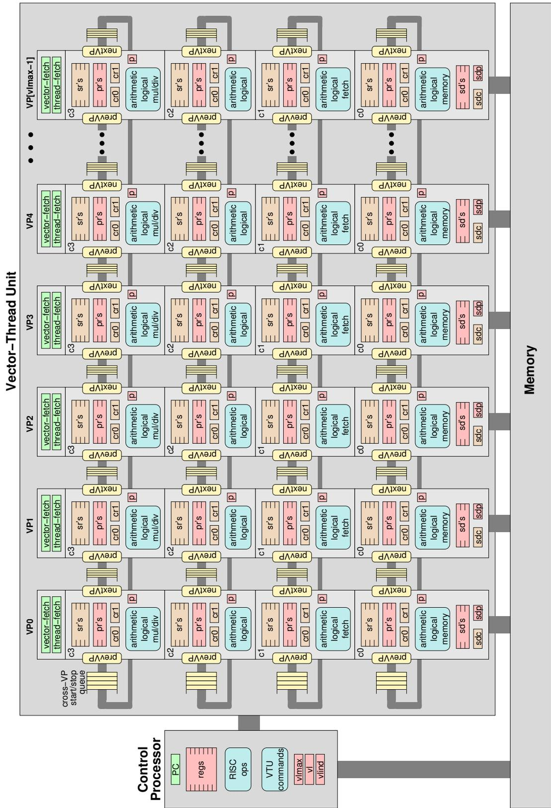
Figure 4-1: Programmer's model for the Scale VT architecture.
