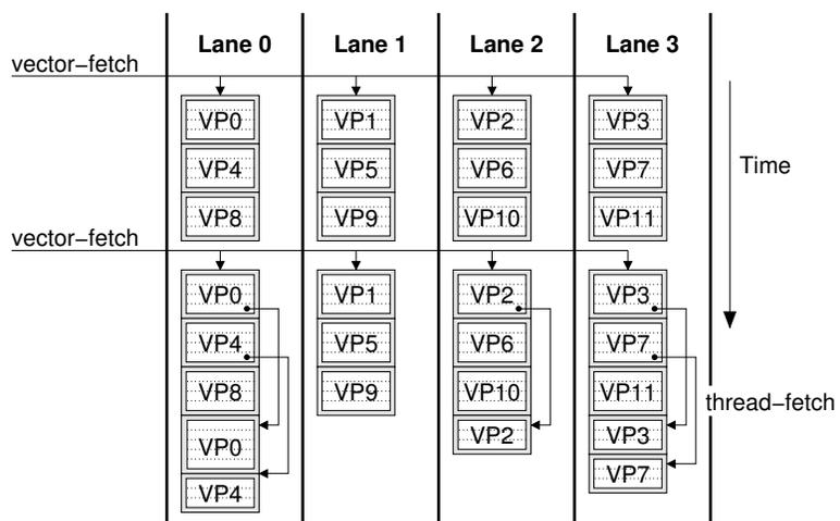
Figure 2-19: Time-multiplexing of VPs in a VT machine.
