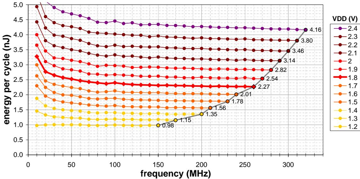
Figure 6-16: Chip energy versus frequency for various supply voltages. All data is for running the adpcm\_dec test program in the on-chip RAM operating mode. For each supply voltage, the maximum frequency point is marked and labeled with the energy value.
