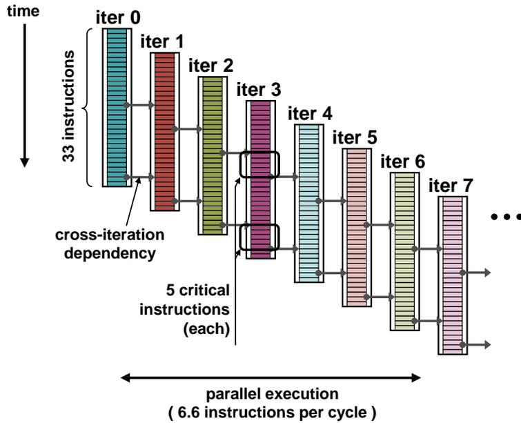
Figure 7-9: Ideal execution of the `adpcm_dec` benchmark, assuming each iteration executes one instruction per cycle. The two cross-iteration dependencies limit the parallel execution to one iteration per 5 cycles, or 6.6 instructions per cycle.
