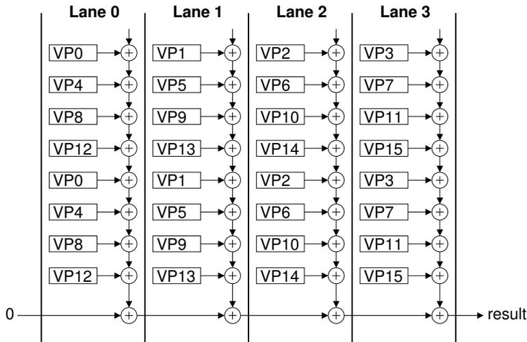
Figure 4-8: Reduction example. The diagram shows a sum reduction accumulated first within 4 lanes, and then the final result accumulated across the 4 lanes.
