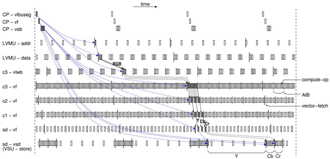
Figure 7-2: Diagram of decoupled execution for `rgbicc` kernel. One lane is shown. The operations involved in a single pixel transformation are highlighted. The control processor would generally be running even further ahead, but the decoupling has been condensed to fit on the figure.
