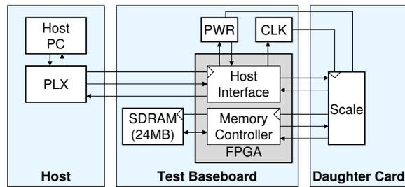
Figure 6-7: Block diagram of Scale test infrastructure.
