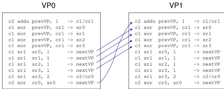
Figure 4-7: Example showing the need for cross-VP buffering. The AIB is shown for VP0 and VP1, and the cross-VP dependencies are highlighted.
