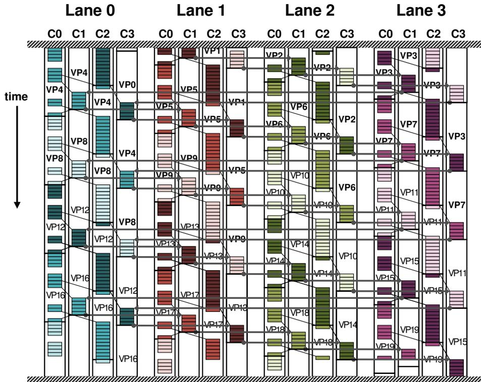
Figure 7-10: Execution of the `adpcm_dec` benchmark on Scale. Each small shaded box represents an individual compute-op. The narrow lines within a lane indicate inter-cluster data transfers, and the thicker arrows between lanes indicate cross-VP data transfers.
