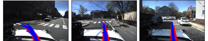
(c) Without IMU inputs, there are overshooting and undershooting predictions even when in smooth motion.
