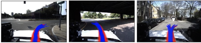
Fig. 7: Demonstrated predicted trajectories with the variational predictor. Left to right: the vehicle is turning right, following roundabout beneath a highway, and facing two options in front of a T intersection.
