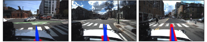
(b) Without CANBUS inputs, there is always motion predicted even when the vehicle is moving.
