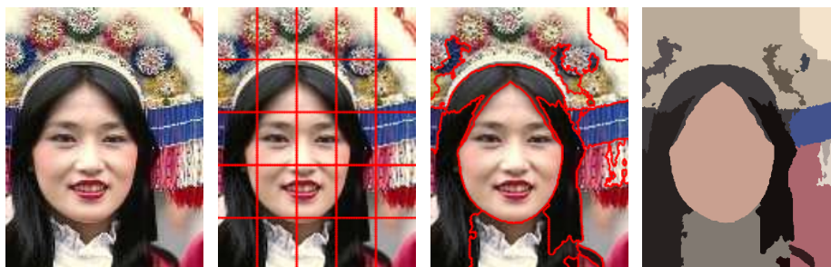
Fig. 7. Segmentation obtained using the Gaussian mixture to model image intensity probability density. Left to right: the original image, the initial contour, region boundaries obtained by our method, regions colored according to their mean intensity values.
