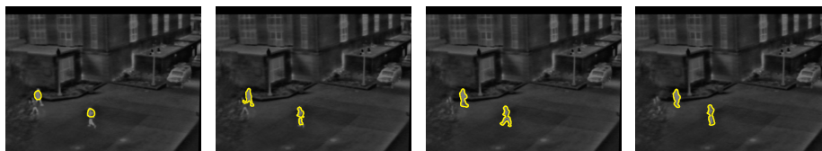
Fig. 6. Tracking in a thermal camera video sequence from a surveillance camera. Yellow contours show the region boundaries in four frames from the sequence. The leftmost subfigure demonstrates the initial contour.
