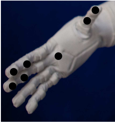
Fig. 5. Robonaut 2 hand. The black dots indicate the contacts used in the experiments.
