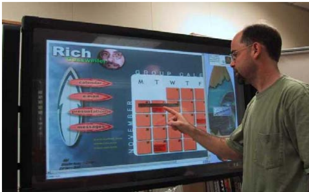
Figure 1. The BlueBoard is a large, interactive display surface offering fast access to personal information with tools for collaboration and small groups of people working side-by-side. The display has a touch screen overlay and a badge reader on the right corner for person identification. Network access is assumed.
