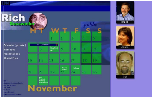
Figure 2. A typical BlueBoard personal display. This kind of content is set up by each user as their "home content." Content displayed on the BlueBoard can be shared with another person by dragging the content (window, image, URL) to their p-con. Here, Rich is showing his home page calendar to Daniel and Alison.
