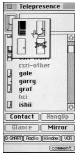
Figure 3.9 The original doors interface allowed users to select from four different door states: open, ajar, closed and locked
