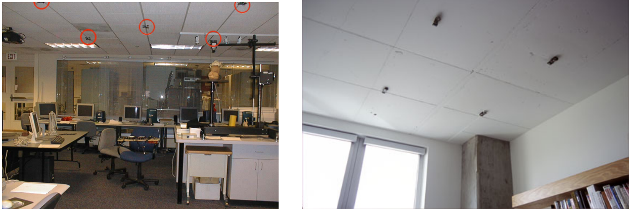
Figure 1.2: Example deployments of Cricket beacons. Multiple beacons may advertise the same space identifier if they are in the same space, but each beacon has a different position coordinate consistent with its location in space.
