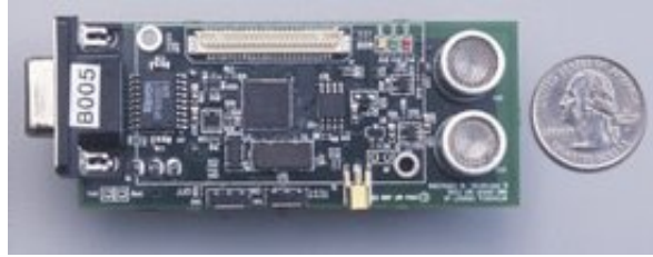
Figure 1.1: A Cricket hardware unit; this unit can function as either a beacon or a listener under software control, and can also be used in a more symmetric way as both listener and beacon.
