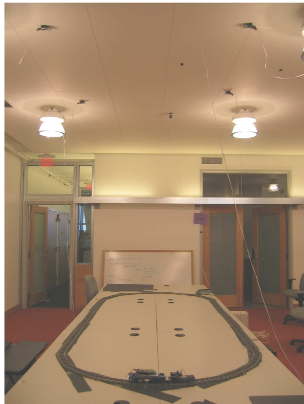
Figure 5: Picture of the experimental setup. The beacons are shown on the ceiling; the cables emanating from the beacons are used in a subset of the active mobile experiments to report distance samples observed by infrastructure nodes.
