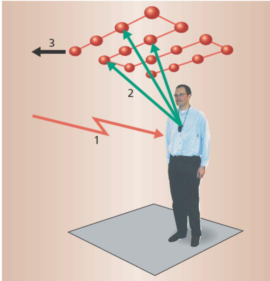
*Figure 1. Operation of the Bat location sensor system. A Bat is triggered over a wireless link (1), which causes it to emit an ultrasonic pulse (2). Ceiling-mounted receivers measure the pulse's times of flight, and a controller retrieves the times of flight (3) over a wired network. The controller uses these measurements to calculate Bat-receiver distances and thus the Bat's 3D position.*
