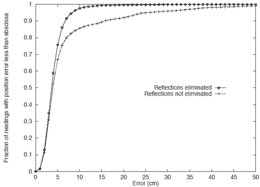
Figure 3. Position accuracy of ultrasonic tracker
