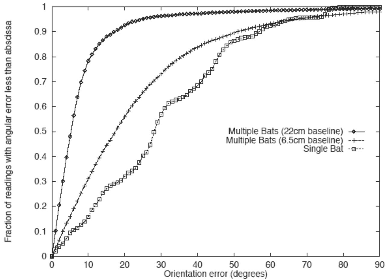
Figure 4. Orientation accuracy of ultrasonic tracker
