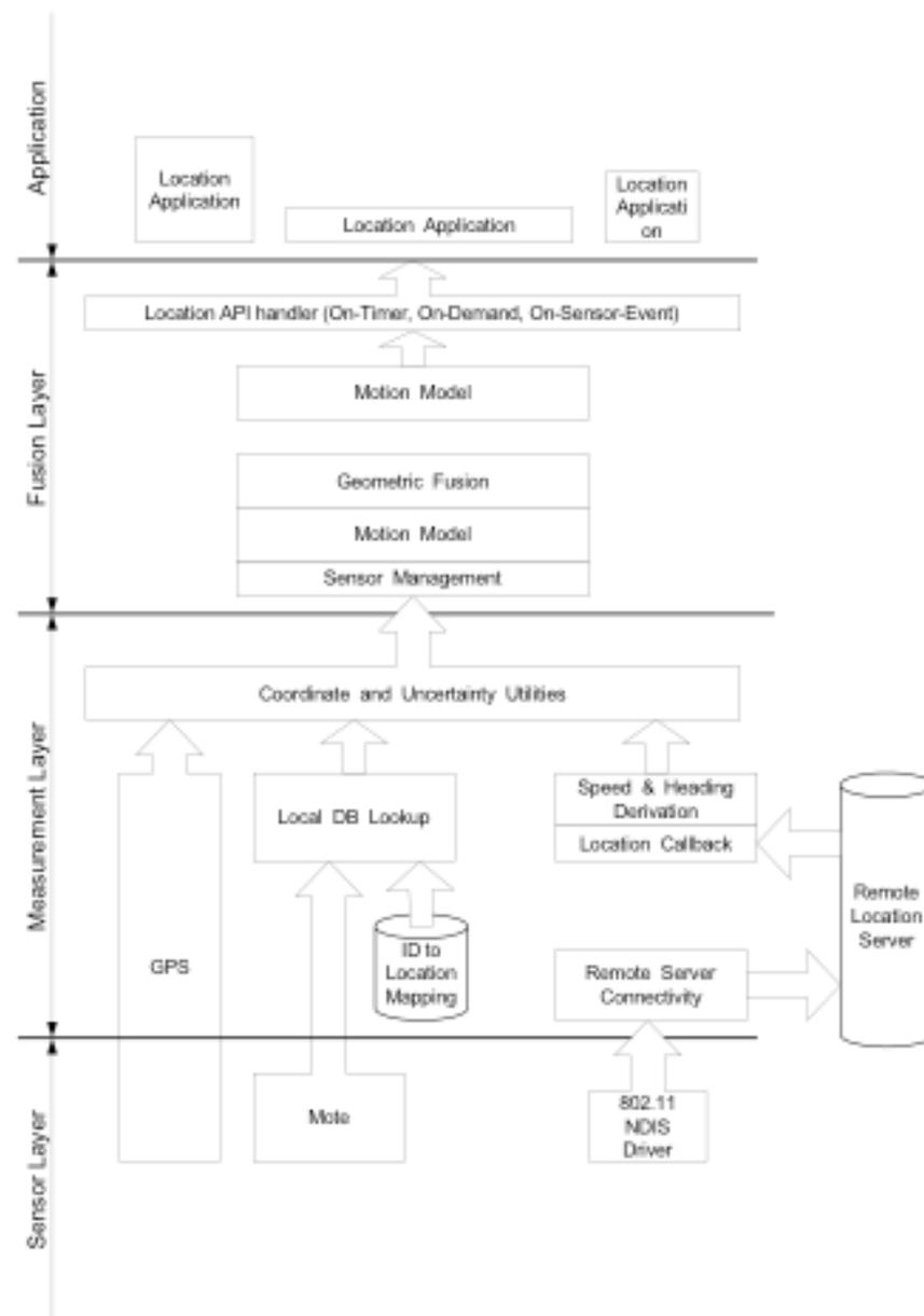
Figure 3. Universal Location Framework block diagram.
