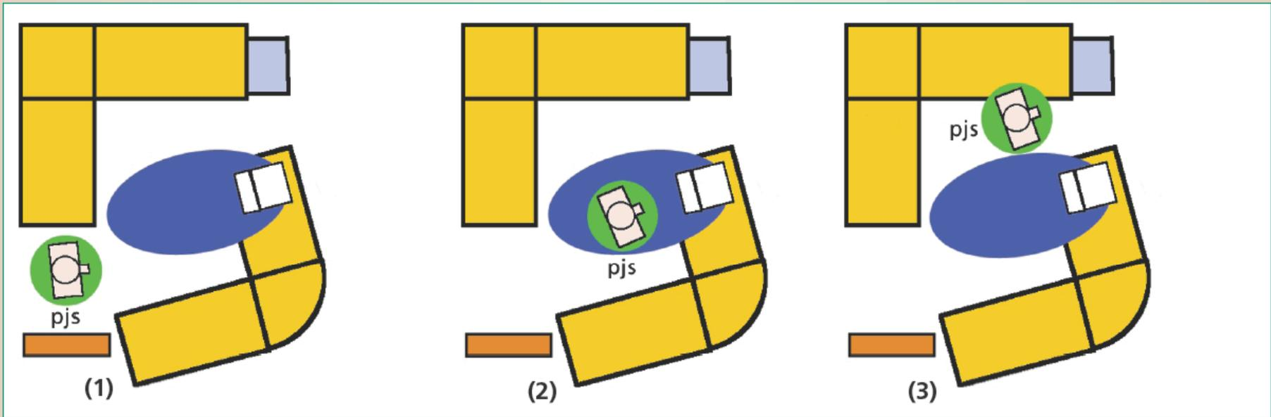
*Figure A. Spatial monitoring application that moves users' desktops around with them. The application registers with the Spatial Monitor (1); as the user (pjs) approaches the display (2) or moves away from it (3), the spatial monitor sends a positive or negative containment event to the application that transfers or removes the desktop to or from the screen.*
