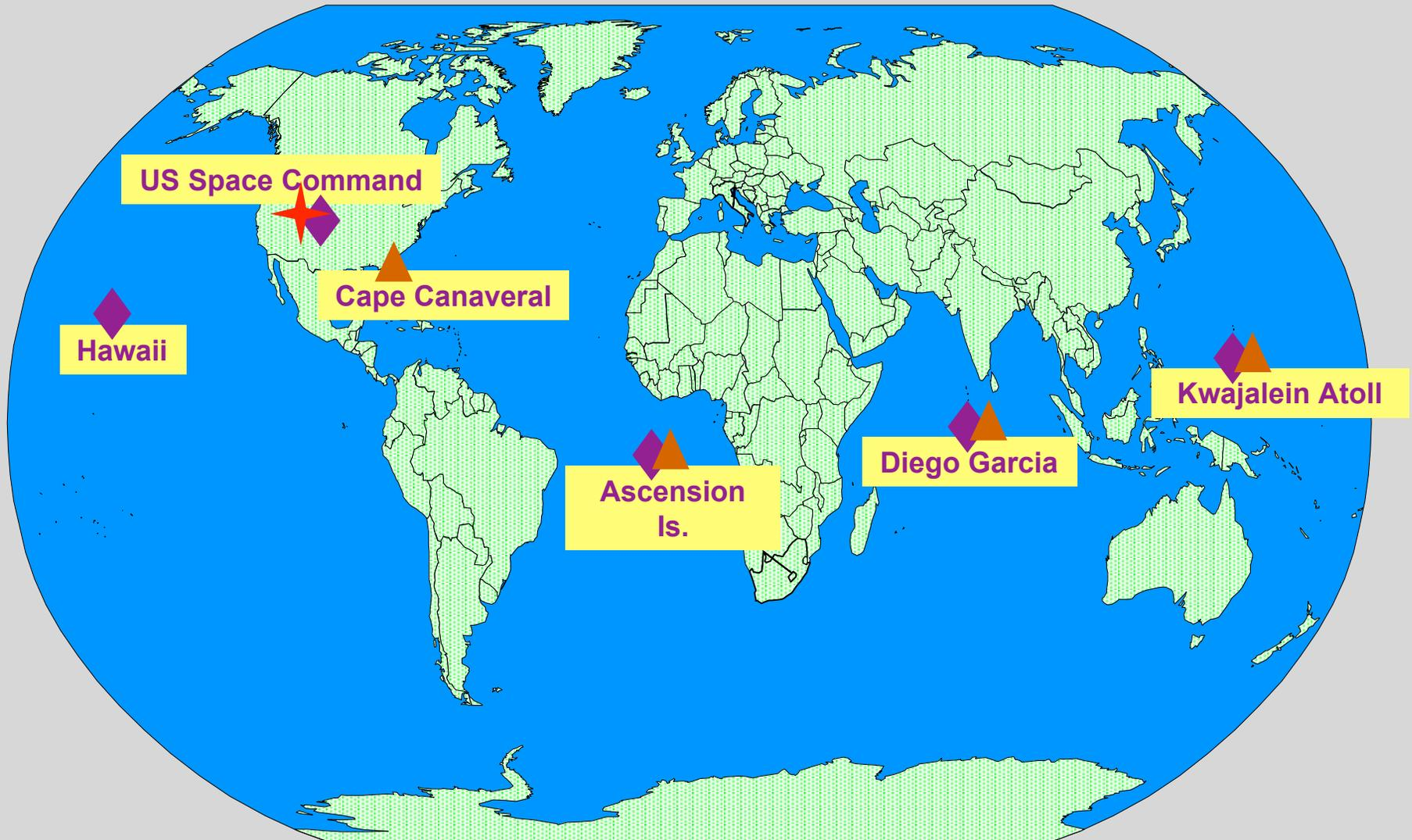
★ Master Control Station    ◆ Monitor Station    ▲ Ground Antenna
