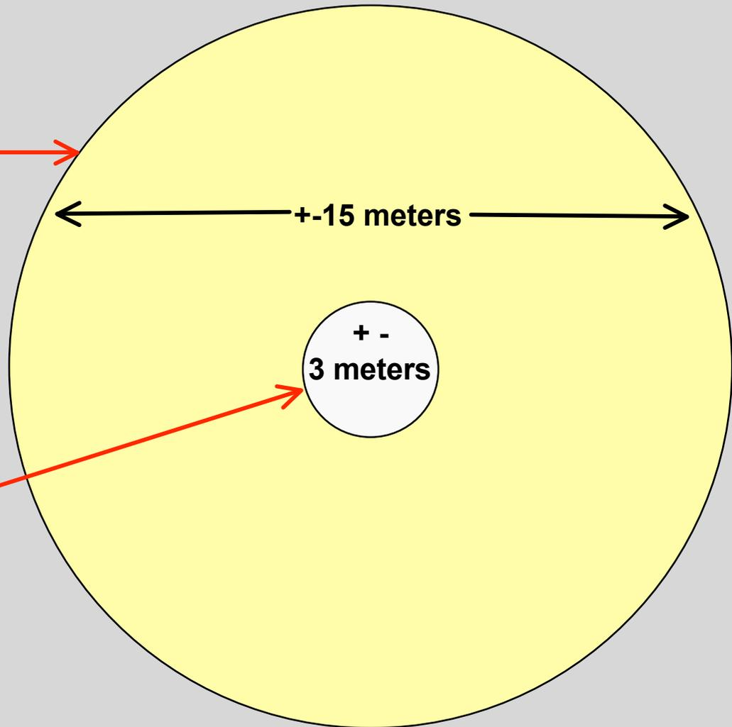
\* Precision depends on good satellite geometry, open sky view, and no user induced errors.
