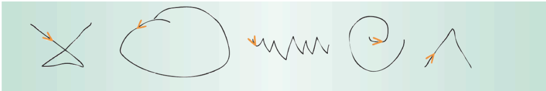
Figure 3. Editing gestures that SILK supports. From left, the first gesture deletes widgets or other objects in the sketch. The next three gestures help inform the recognition process: group objects, ungroup objects, and cycle to the next best inference. The last gesture lets the designer insert typed text or replace a text squiggle with typed text. The arrows show the direction to draw the gestures for best recognition.
