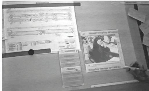
Figure 3.12 Ariel lets construction engineers access the media space and a hypermedia annotation item via paper engineering drawings. The user selects the media space option from the control section of the paper engineering drawing (upper left). Ariel projects a menu and the user selects Glance with the graphics tablet pen, which establishes a three-second connection
