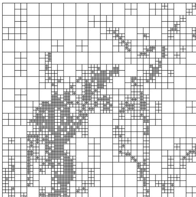
Figure 4: Quadtree partitioning for figure 3, 2812 ranges
