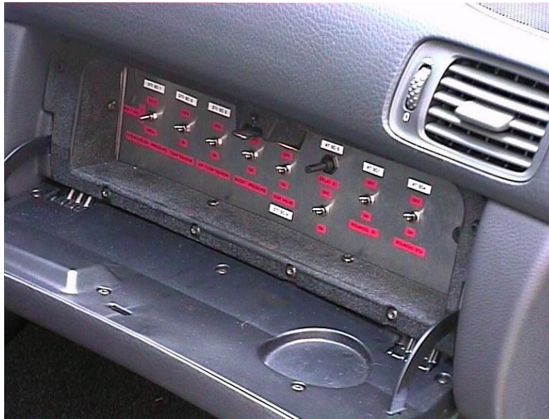
Figure 8.2: The glove compartment of the Volvo Demonstrator Car which contained the switchboard for controlling the built-in faults
