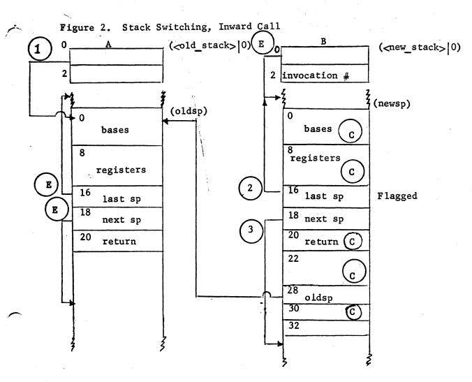
Stack A belongs to the ring of the calling-procedure (old\_ring), stack B to the target procedure (new\_ring).
