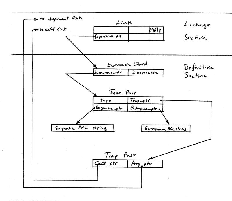
Figure 2: The Structure of a link
