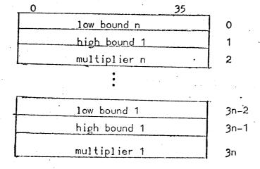
The bounds are derived directly from the declared bounds of the argument. The multipliers are computed from the bounds and the element size. Multipliers of packed arrays are expressed in bits, multipliers of non-packed arrays are expressed in words.
