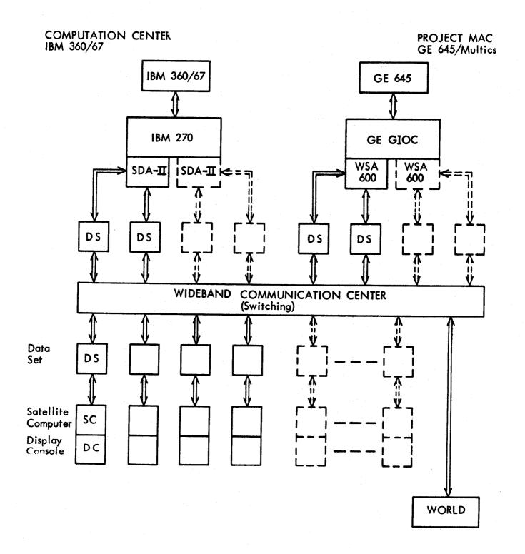
FIG. 1 PLAN FOR WIDEBAND COMMUNICATIONS WITHIN MIT
