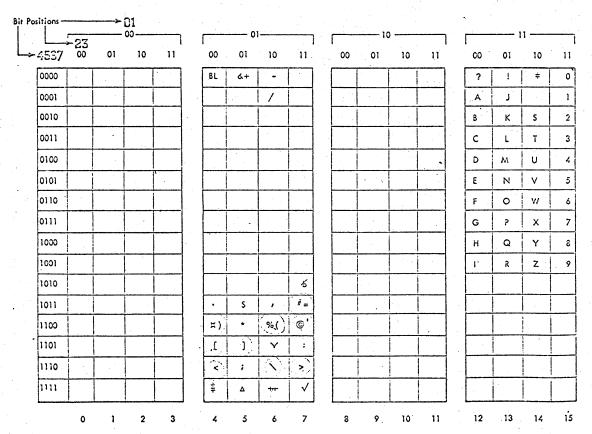
Figure 16. Translation Chart - Extended BCD Interchange Code to BCD Interchange Code
