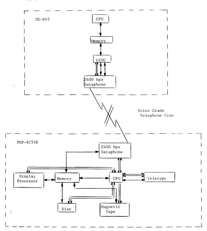
(Single lines represent data transmission; double lines represent transmission of status information and interrupts)
