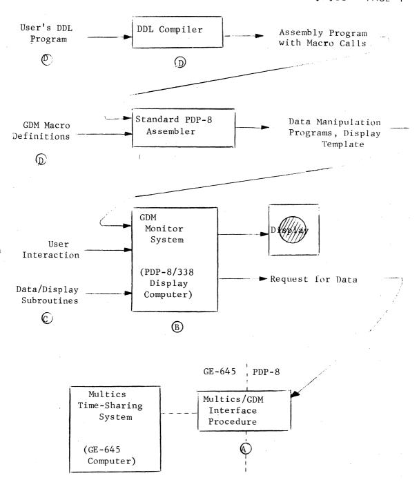
$\label{eq:figure 1} \mbox{ Figure 1}$   $\mbox{GDM Subsystem Interactions}$
