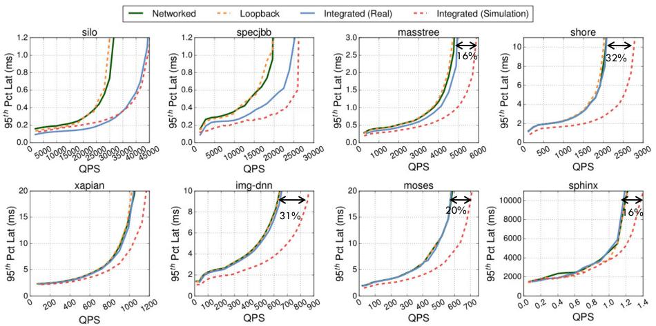
Performance difference between real and simulated systems well within usual simulation error bounds
