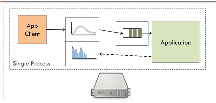
Application and client integrated into a single process
