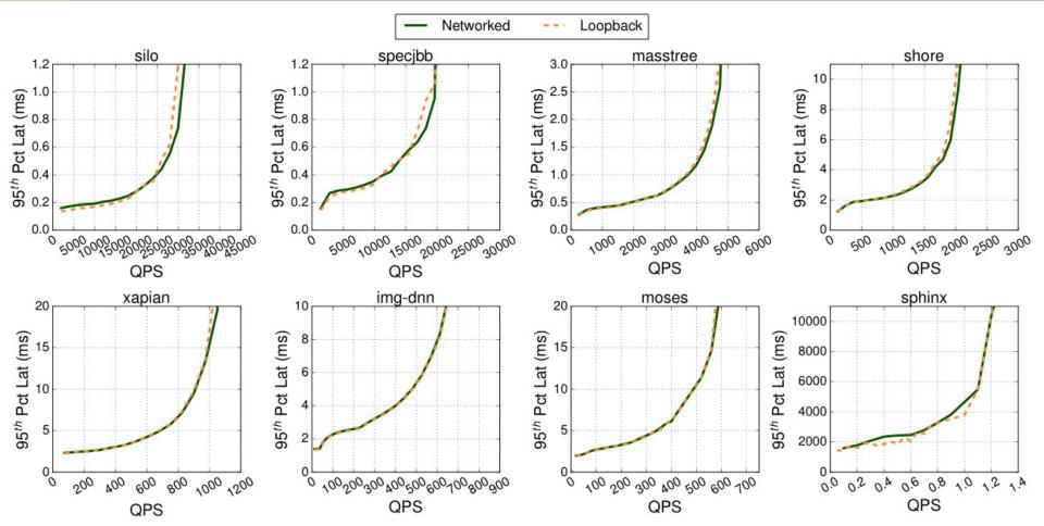
Loopback and Networked configurations have near-identical performance
