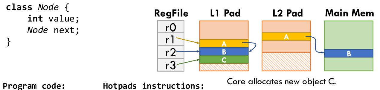
Node C = new Node(); alloc r3, type=Node
