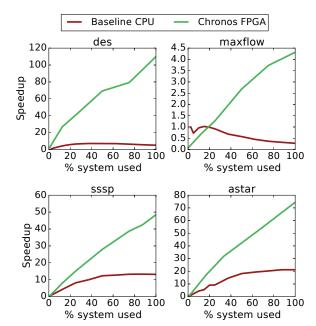
**Figure 10.** Scalability of Baseline CPU and Chronos implementations of the ordered algorithms. For CPU, 40 threads = 100% system. For Chronos, 100% corresponds to the number of tiles in Table 3. Speedups are normalized to the serial CPU version.
