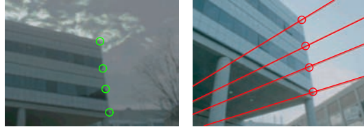
Figure 39. AmesCourt Epipolar Geometry. Point features and corresponding epipolar lines for a typical node pair in the AmesCourt set.
