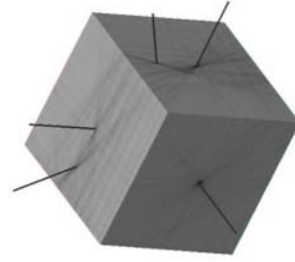
Figure 7. Hough Transform for VP Detection. A Hough transform of real line data. The HT algorithm accumulates all lines in a given node, then finds peaks in the antipodally-symmetric accumulation space, implemented as three faces of a unit cube.
