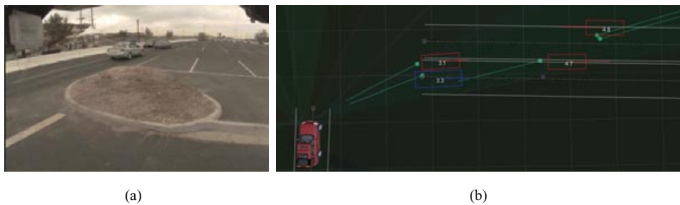
Figure 12. Radar tracking three vehicles. (a) Front right camera showing three traffic vehicles, one oncoming. (b) Points: Raw radar detections with tails representing the Doppler velocity. Rectangles: Resultant vehicle tracks with speed in meters per second (rectangle size is simply for visualization).
