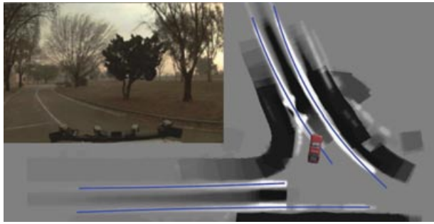
Figure 17. Our system constructs a centerline evidence image using road-edge and road-paint detections. Lane centerline candidates (lines) are identified by fitting parabolic segments to the ridges of the image. Front-center camera is shown in top left for context.
